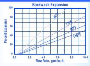
**Backwash:** After each cycle the resin bed should be backwashed at a rate that expands the bed 50 to 75 percent. That will remove any foreign matter and reclassify the bed. The graph above shows the expansion characteristics of Pure PC003ID in the sodium form.
